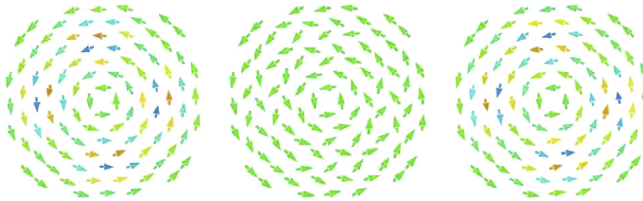
Fig. 16. (Color online) Second highest-frequency vortex mode. This mode has a d-wave symmetry.
